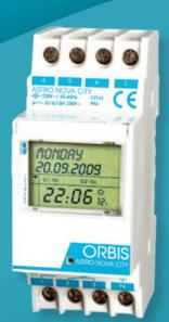
The ASTRO NOVA CITY is a time switch which controls the switching ON/OFF of any lighting circuit or installation according to the dawn and dusk of the area. The different areas are programmed using an easy text menu. The times are set using the main cities of your country and therefore you simply choose the city closest to you. The installation uses Din rail without the need of any external wiring out of the cabinet; also, it does not require any maintenance to maintain the accuracy.
